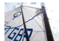
Fig.1 Head tie too loose
