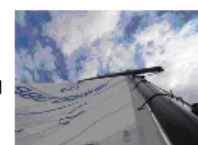
Fig.3 Luff too tight
